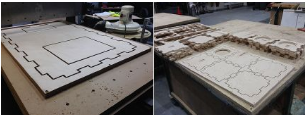
Figure 23: Build Process - Cubes & Satellite Speakers
